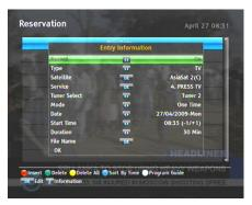
To add a timer recording, select the Recording > Reservation menu; then the timer list will be displayed. To add a new timer event, press the [5] button, and a box like the left figure appears. Take the following steps:
