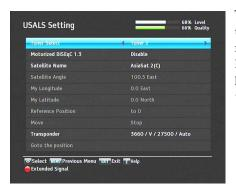
To use the USALS protocol, select the Installation > USALS Setting menu. You should see a screen like the left figure. At first you have to set the Motorized DiSEqC 1.3 option to Enable.
