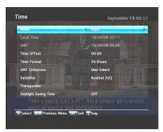
Select the Settings > Time menu. You should see a screen like the left figure. You can set the clock manually or use the time signal, Greenwich Mean Time (GMT), carried as part of the digital television broadcast. To use Greenwich Mean Time, take the following steps:
