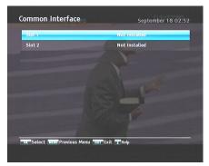
To view the information about the module and subscription card which is inserted into the digital receiver, select the Information > Common Interface menu. You should see a screen like the left figure.
