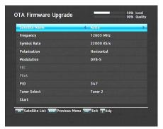
You can get a new firmware over the air. Select the Installation > Firmware Upgrade > OTA Firmware Upgrade menu. You should see a screen like the left figure. Selecting the Start command starts firmware update.
