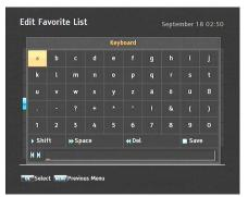
You can move the highlight key horizontally with the ② and ③ buttons and vertically with the ③ and ② buttons. Pressing the OK button on a key enters its letter in the input line.
