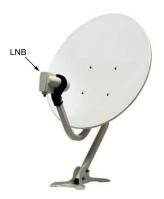
The LNB (Low Noise Block converter) is used to take a wide band of relatively high frequencies, amplify and convert them to similar signals that is carried at a much lower frequency, which is called Intermediate Frequency (IF). High frequencies from satellites are converted into 950 to 2150 MHz by a LNB.
