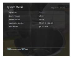
You have to check the firmware information of your digital receiver before downloading a new firmware. Select the Information > System Status menu. You should see a screen like the left figure. Remember the number of the System ID item, and download the latest firmware with the same system identification.
