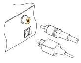
To enjoy Dolby digital audio, your television or audio-video receiver must be able to decode Dolby digital audio, and you need to obtain an S/PDIF cable. If you want to use the COAXIAL connector, prepare a coaxial S/PDIF cable (RCA cable); otherwise, to use the OPTICAL connector, prepare an optical S/PDIF cable.
