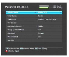
To use the DiSEqC 1.2 protocol, select the Installation > Motorized DiSEqC 1.2 menu. You should see a screen like the left figure. At first you have to set the Motorized DiSEqC 1.2 option to Enable.
