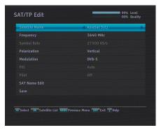
You can change attributes of a transponder. Select the Installation > SAT/TP Edit menu. You should see a screen like the left figure. To change the information of a satellite entry, perform the following steps:
