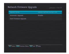
Select the Installation > Firmware Upgrade > Network Firmware Upgrade menu. You should see a screen like the left figure.
