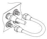
Whatever sort of connection you have between the digital receiver and the television, you need to connect the digital receiver to the antenna so that it can receive digital television services. Connect the antenna cable to the LNB 1 IN connector on the back panel of the digital receiver. Also, you must ensure that there is a connection to both the LNB 1 IN and LNB 2 IN connectors on your digital receiver, so that both tuners work properly.
