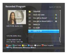
Select the Recording > Recorded Program menu or alternatively press the button to display the recorded programme list. The file information is comprised of the following elements: file number, filename, recording time, playing duration, file size and so on.
